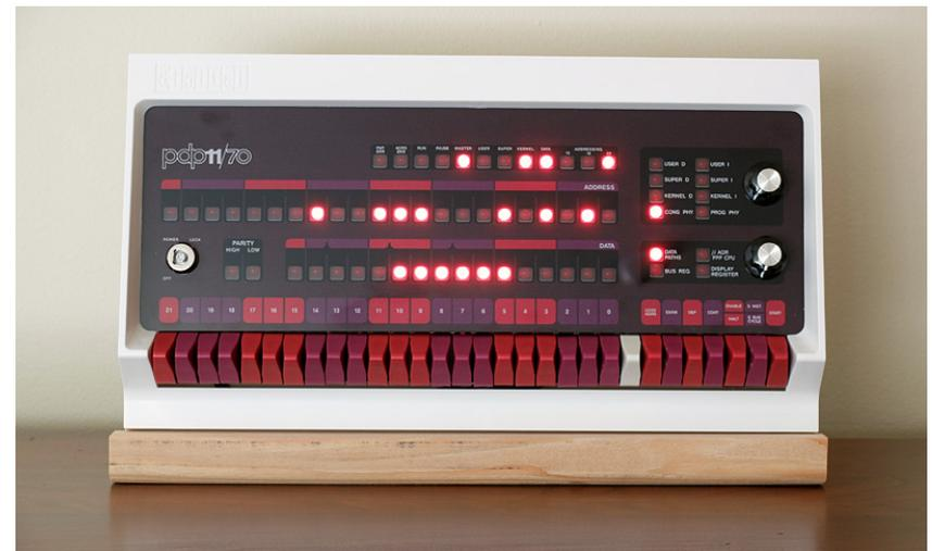
DEC PDP11/70 front panel replica (3D printed) connected to a Raspberry Pi running a PDP11 emulator
