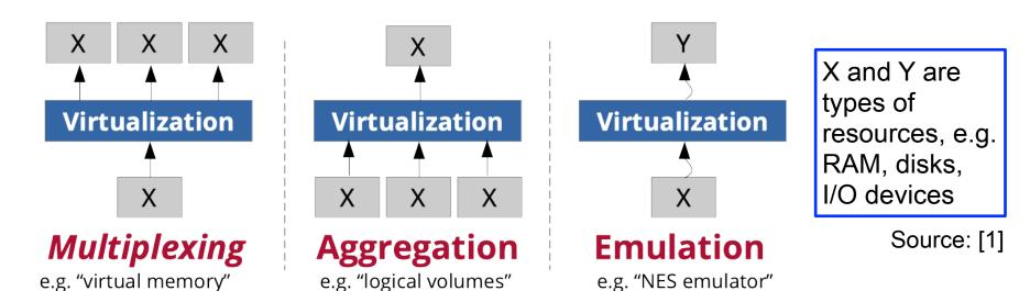
This construction principle can be replicated on different layers and for different resources
