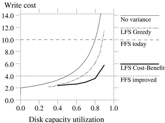
**Figure 7 — Write cost, including cost-benefit policy.** This graph compares the write cost of the greedy policy with that of the cost-benefit policy for the hot-and-cold access pattern. The cost-benefit policy is substantially better than the greedy policy, particularly for disk capacity utilizations above 60%.
